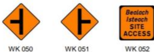
Figure 3.1: Temporary Traffic Signage Examples
